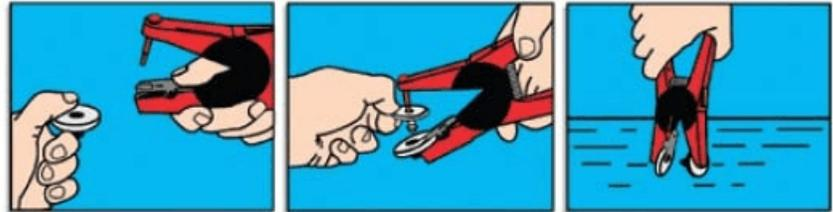
1. To load, depress spring clip and insert the female EID tag. Ensure that the raised portion of the tag, which encloses the transponder chip, is placed in the open portion of the jaws.
